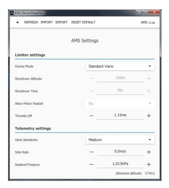
AMS settings. Every time you make any change in the configuration, the new value is immediately transferred to the device and saved to memory. There is no need for additional confirmation.
