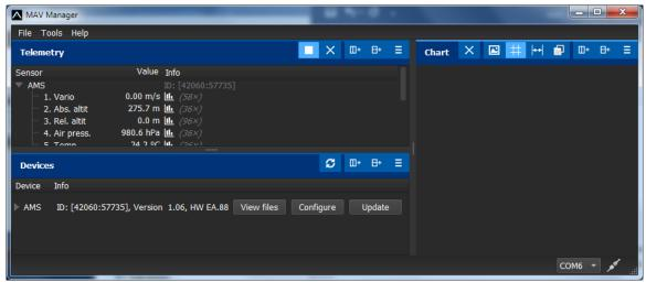
Connect the AMS to your PC using the USB interface. The device will be automatically detected by the MAV Manager. The device properties are available after pressing the "Configure" button.
