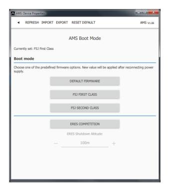
Setting competition modes using the "Boot Mode" menu. After confirming the mode change, the AMS must be disconnected from the power supply.
