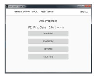
The initial sensor menu shows the main device mode and links to alter the competition mode or modify the sensor settings.
